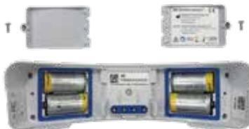
3. Install the four CR123A batteries provided. Ensure the batteries are inserted as indicated in the HeartSine Gateway battery compartment.
